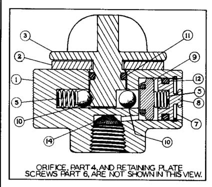
NO. 124 MGM CONTROL VALVE IS AN ALL STAINLESS STEEL CONTROL VALVE DESIGNED PRIMARILY FOR USE ON SLIP TUBE LIQUID LEVEL GAUGES.
